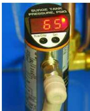
The gas mixer utilizes a solid-state pressure switch to control the surge tank pressure. A digital readout of the pressure is built into the switch. Both the sensing element and electrical switch are solid-state. An LED indicator shows when the surge tank is filling. Use of this pressure switch virtually eliminates the most common cause of gas mixer failure.
